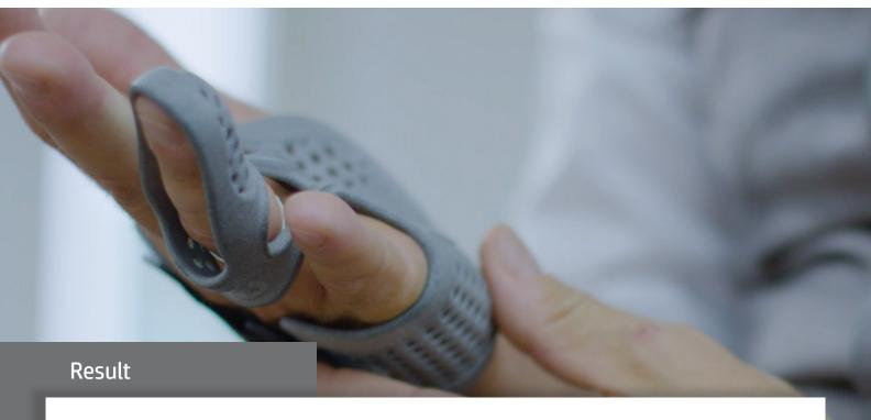
With HP MJF technology, OT4 is now able to manufacture products without the need to apply expensive post-processing. Parts produced with HP MJF have the same properties in x, y, and z directions, which means the build chamber space can be maximized for each production job and with optimal nesting; this, in turn, can help drive down costs.
